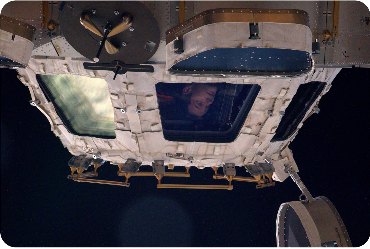
The Cupola as seen from outside
