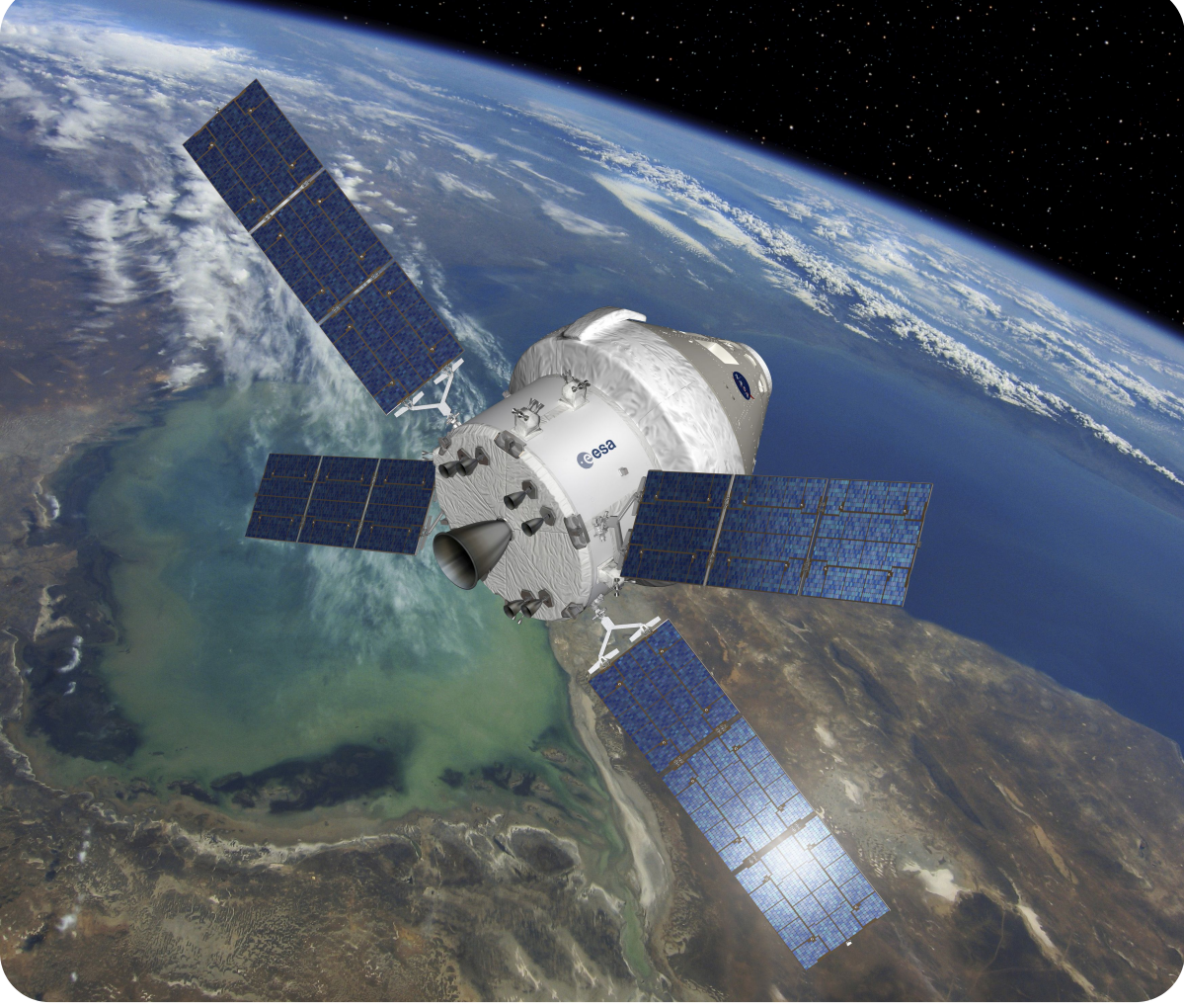
This is what the craft will look like when it is in space! Orion's crew capsule looks like a large nosecone at the front. ESA's European Service Module is at the back, with four solar panels stretched out to collect sunlight.
