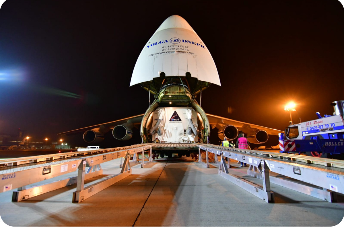
The nosecone of the Antonov An-124 was opened in order to load the European Service Module
