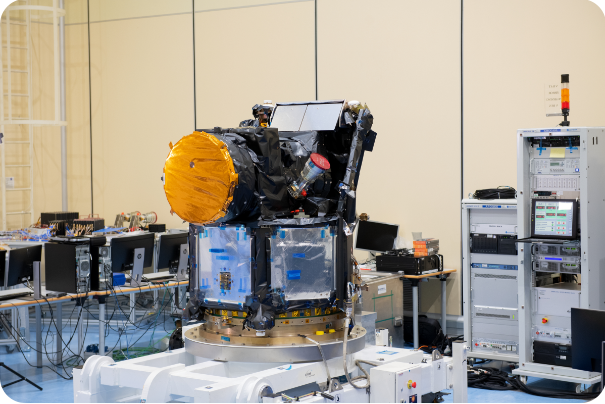
The CHEOPS satellite being tested before launch. It is 1.5 metres long, and weighs 280kg. Copyright: ESA - S. Corvaja Access the image
